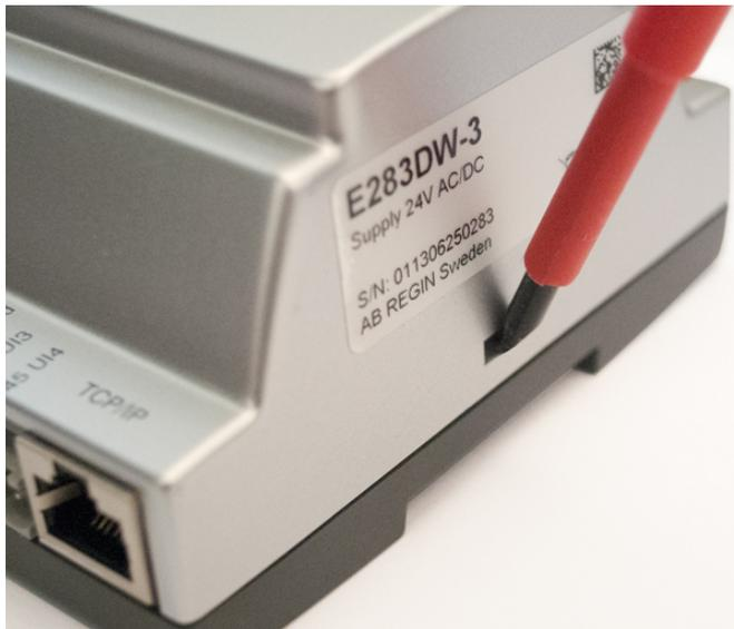
Remove the cover by pressing down the locking torques at the edge of the cover using a small screwdriver, and at the same time pulling the edges outwards.
