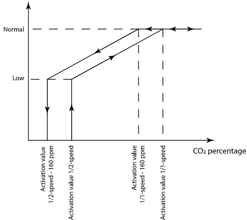
When used with 2-speed fans they will start using reduced speed when the CO<sub>2</sub> value rises above control value one and switch to normal speed when the CO<sub>2</sub> value reaches control value two. The fans will stop when the CO<sub>2</sub> value falls 160 ppm below control value one.
